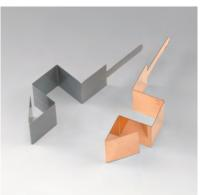
Test piece for the bent cathode plating test using a Haring cell.
