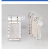
Diaphragm-type Cartridge for insoluble anodes. Both single-sided type(B-77-P30) and double-sided type(B-77-P30-1) are available. Standard product is a neutral type diaphragm (for copper sulfate plating). Anion type and cation type are acceptable as special order products. For details, please contact us. It is also possible to make a cartridge for tanks other than Haring cell. Please inform us desired types and size.
