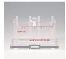
Dedicated tank for measuring macro throwing power. Also convenient for other experiments and trial plating to micro parts. Various busbars, anode plates, and jigs, recommended to make experiments easier to perform, are available.
